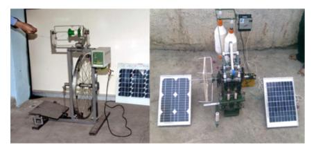
Four out of our twenty power looms have been upgraded with solar powered motors. Spinning and reeling is completely processed either manually or with solar machines. This makes 70% of our spinning and weaving operation zero-carbon.
